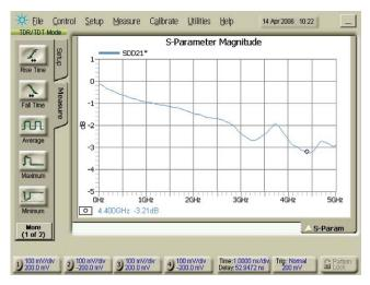
Figure 11. Insertion Loss
