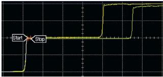
13. If the markers are located on the incident (first) step response as shown above, you must move them to the reflected (second) step response. Adjust the horizontal position knob to move the incident step response off the left edge of the display. The markers will automatically move to the reflected step response.
