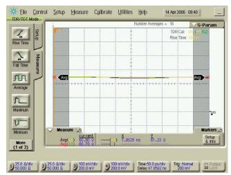
Figure 5. Common Mode Impedance
