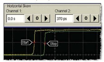
17. Next, adjust the **TDR Skew** setting. Entered values represent the percentage of available adjustment range. Try entering a positive 20% value for the channel with the longest path and a negative 20% value for the channel with the shortest path. Adjust as needed to adjust the mean delta time value to as close to a value of zero as possible.
